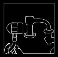
Do not over twist or pretzel the arm or spin the sensor head; you risk breaking the wires that connect from the sensor to the body. Use up, down, left and right motions to gently adjust the arm to your desired placement.
